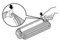
**4b** turn the two levers on the toner cartridge with firm pressure.
